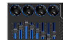
Four encoders and eight faders make the event operations amazingly convenient. Also, the encoders and faders can be bound with external MIDI functions for volume adjustment and more.
