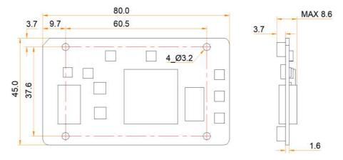
Tolerance: ±0.3 Unit: mm
